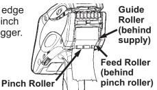
**10.** Turn on the printer and put into load mode.
