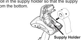
Feed the supplies under the applicator roller and over the label deflector.
