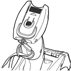
4. Pull the strap and guide the thin end's loop over the plastic piece in the middle of the strap.
