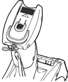
2. Take the thin end of the safety strap and push it through the loop at the bottom of the printer handle (near the battery compartment).
