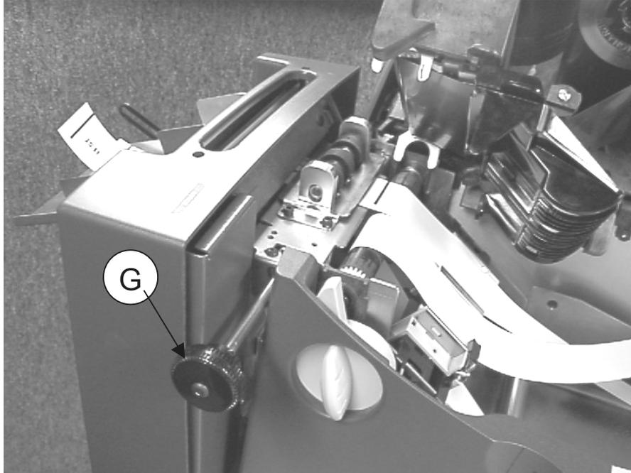
10. Insert the label strip into both sides of the supply guide. Adjust the supply guide by moving the right guide in or out, depending on the stock width. The label strip should be in the guide slots on the inner edges of the strip and under the sensor at the back right of the guide. Adjust the supply guide so that it just matches the width of the inner strip. The outer strip will be slightly loose.
