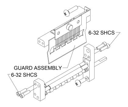
9. Re-attach the nip roller assembly to the machine using the (2) 10-32 round head, mount screws from step 1. Re-attach the 20T drive gear (inside back cover - from step 1 on page 17). Re-attach the stacker. Plug the stacker in and turn the machine on.
