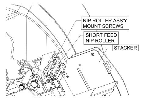
2. Dis-assemble the short feed nip assembly. Remove the (2) 6-32 SHCS from each roller bracket end, and remove the (4) rollers. Note: It is not necessary to dis-assemble the guard assembly or remove the springs. (shown for location and orientation).
