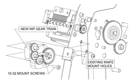
3. Test that feed knob turns freely by hand. Check that all steps have been done correctly. Check that all nip rollers turn freely when feed knob is rotated. If a bind detected, adjust gear train mounting screws (shown in previous step).
