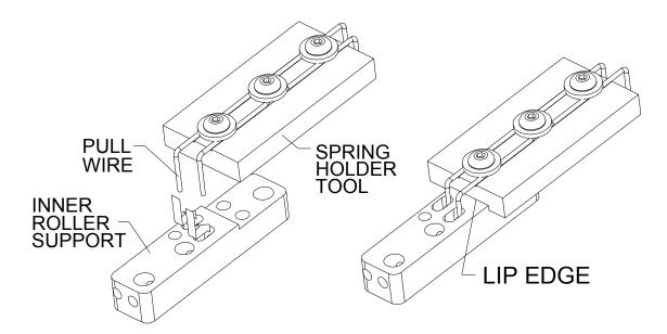
5. Install all (4) rollers into the inner roller bracket. Once all four are seated correctly, remove the spring holder tool.
