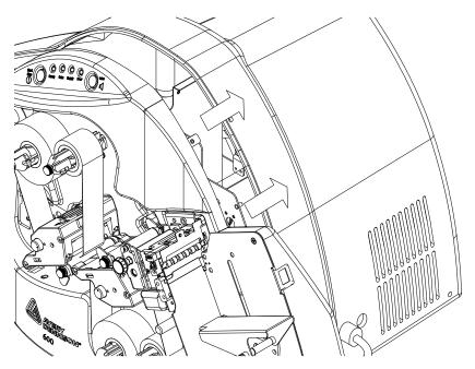
2. Remove old nip assembly by first loosening set screw on old nip drive gear and removing. Loosen mount screws and pull old nip assembly out from front of machine.
