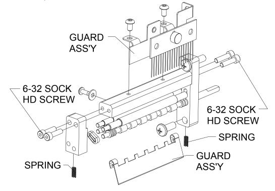
3. Set the smooth rollers aside. Remove the old O ring belts from the two knurled rollers. Replace with new O ring belts.
