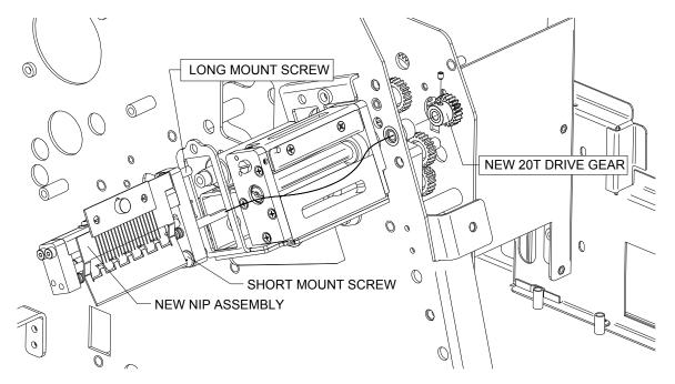
2. Install new nip gear drive train as shown below using the (2) kit provided 10-32 mount screws. Use existing knife mount holes in frame to mount gear chain.
