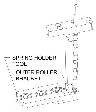
8. Re-assemble short feed nip roller assembly. Make sure inner and outer roller brackets are square with respect to each other (not twisted).
