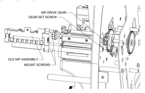
3. Remove old 22T idler gears from old nip drive chain and discard.
