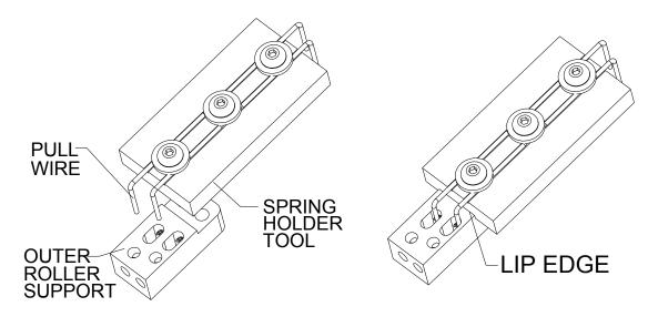
7. Assemble both inner and outer roller brackets with rollers by seating all (4) rollers into the outer roller bracket. Once seated, remove the spring holder tool.
