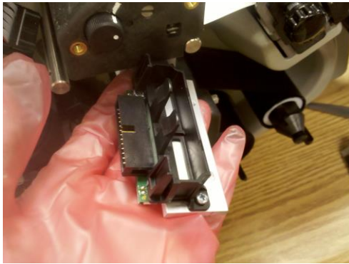
Figure 17c. Print Head Assembly – Removed
