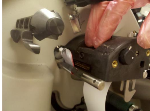
Figure 17b. Two Tabs on Print Station – Depressed
