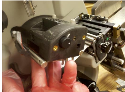
Figure 17d. Inserting Print Head Assembly
