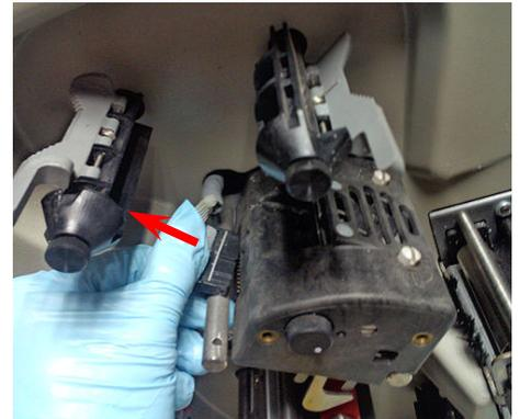
5. Press the two grey tabs on the top of the print station. Reach underneath and remove the print head from the print station.
