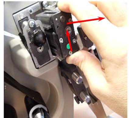
5. Clean the knife with alcohol and cotton swab. Tap the knife on a hard surface to remove cut pieces.
