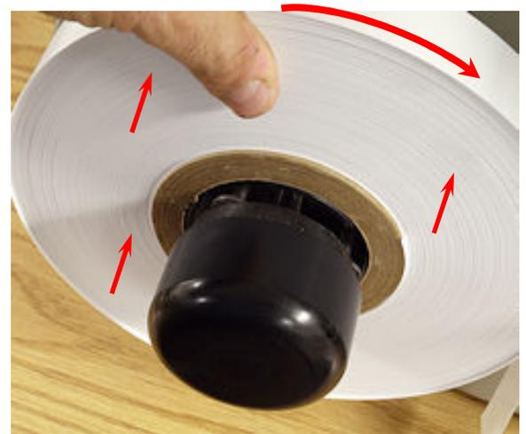
5. Rotate the **Stock Arbor Knob** clockwise quickly to extend the fingers that hold the stock.
