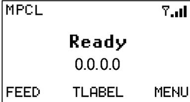
The printer's display shows the antenna symbol when the printer is connected and ready to receive data.
