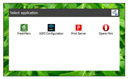
3. Press WIFI Configuration. The Summit Client Utility (SCU) main screen appears. Drag the keyboard out of the way.
