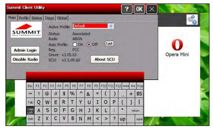
The main screen shows the active profile, current wireless status (Down, Disabled, Not Associated, Associated, or Authenticated), the radio type, the regulatory domain, and the driver version. From the main screen, you can also log in as administrator to make changes to radio settings, and disable or enable the radio.
